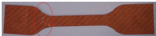
Figure 7. Fracture Region in the specimen
